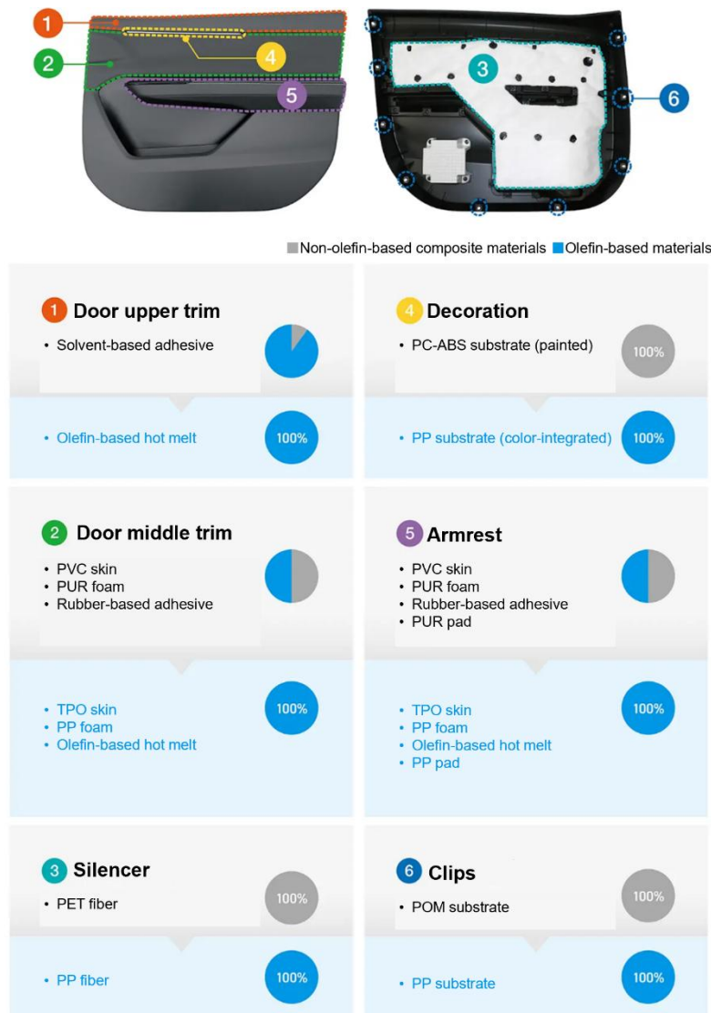
Figure 2: Case study on monomaterialization from composite materials to olefin-based materials
