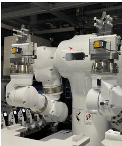
Figure 4: Maholo humanoid robot for cell culture automation
