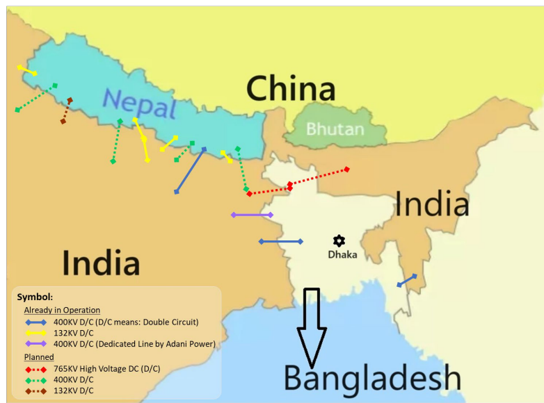
Figure 3: Cross-border power grid between India, Bangladesh, and Nepal and its development plan
