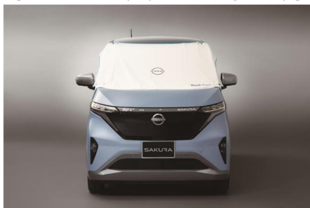
Figure 3: Sunshade (left) and half-body cover (right) using radiative cooling metamaterials
