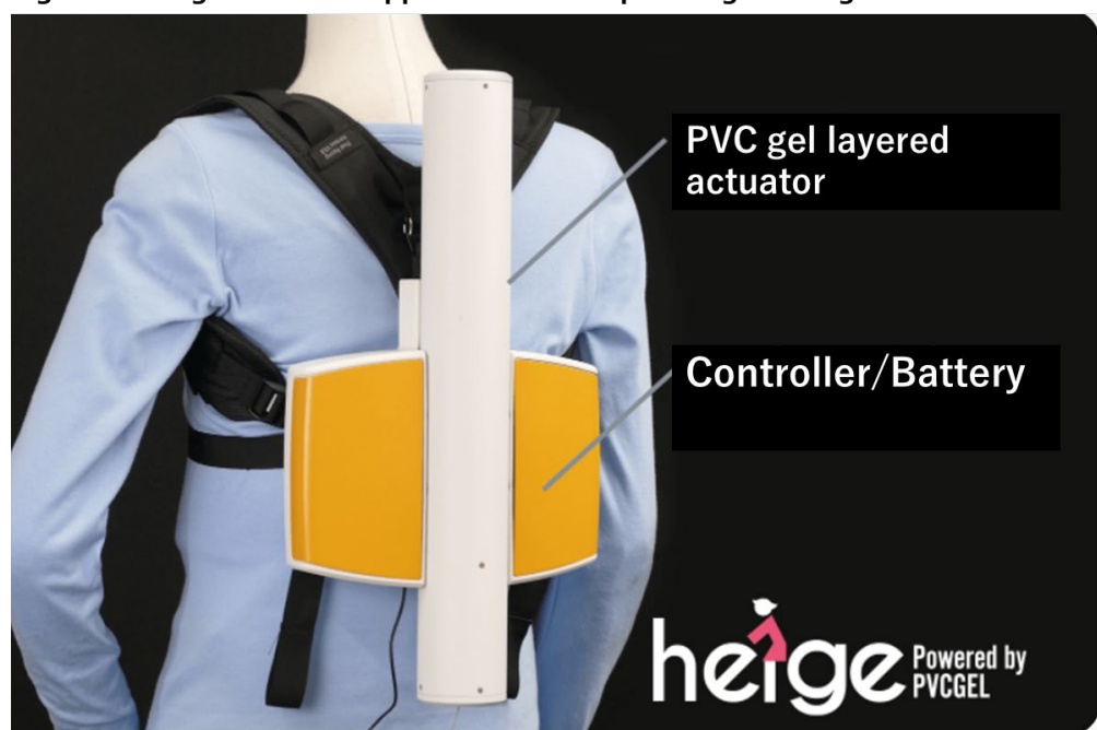
Figure 4. Heige LS back support wear incorporating a PVC gel actuator
