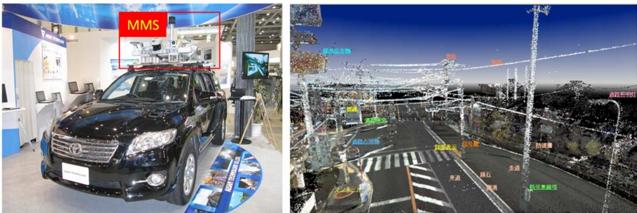
Fig. 2: Vehicle with MMS and 3D Data Obtained from MMS
