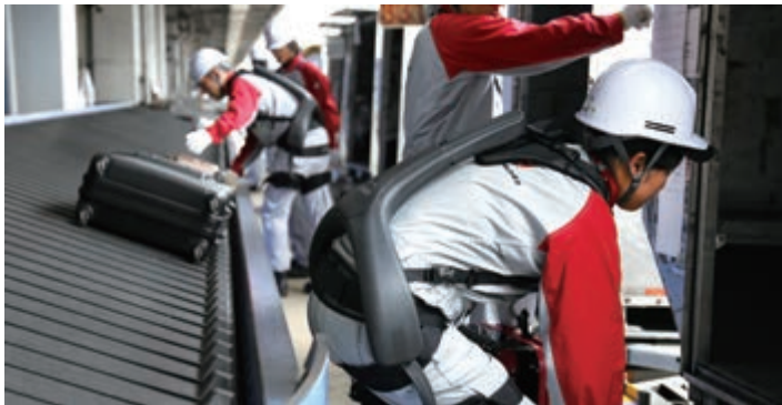
The "ATOUN MODEL Y" introduced for airport ground handling tasks
