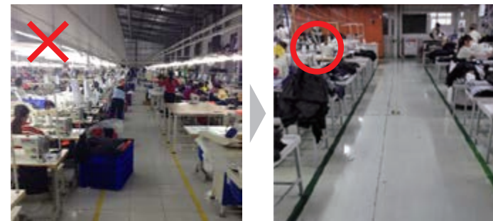
Ensuring safe aisles
