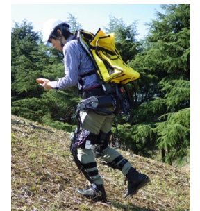
ATOUN is undertaking joint development of powered suits for use in the forestry sector that can be used for walking on slopes, etc., in collaboration with Sumitomo Forestry Co., Ltd., the Forestry Research and Management Organization’s Forestry and Forest Products Research Institute, and Nara Institute of Science and Technology
