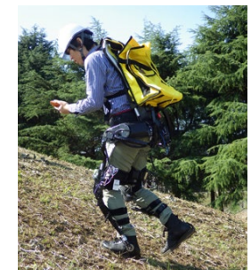
ATOUN is undertaking joint development of powered suits for use in the forestry sector that can be used for walking on slopes, etc., in collaboration with Sumitomo Forestry Co., Ltd., the Forestry Research and Management Organization's Forestry and Forest Products Research Institute, and Nara Institute of Science and Technology
