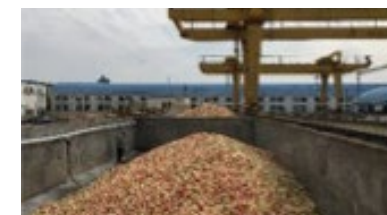
Apple fruit transportation equipment that uses water currents to deliver apples into the factory
