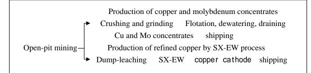
Notes: (1)Dump-leaching means a process to extract (leach) copper by sprinkling sulfuric acid over a pile of uncrushed copper ore.
