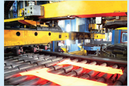
Hot stamping has high potential for automobile weight reduction that leads to reduced GHG emissions.
