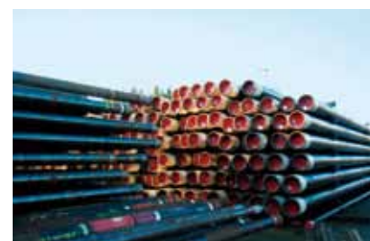
Oil well castings used for production activities in oil and gas fields
