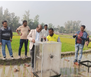
Gas sampling at the project site
