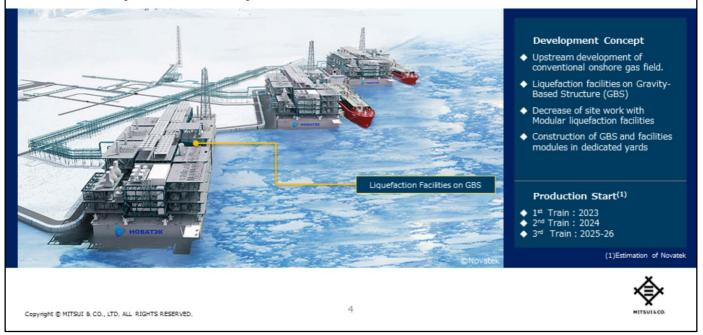
This project operates integrally from upstream gas field development to LNG production. The natural gas produced at the onshore Utrenneye gas field will be delivered via pipelines to the liquefaction facility, where it will be liquefied and then exported. The gas field being developed is conventional and onshore, which contributes to keep drilling costs lower.
